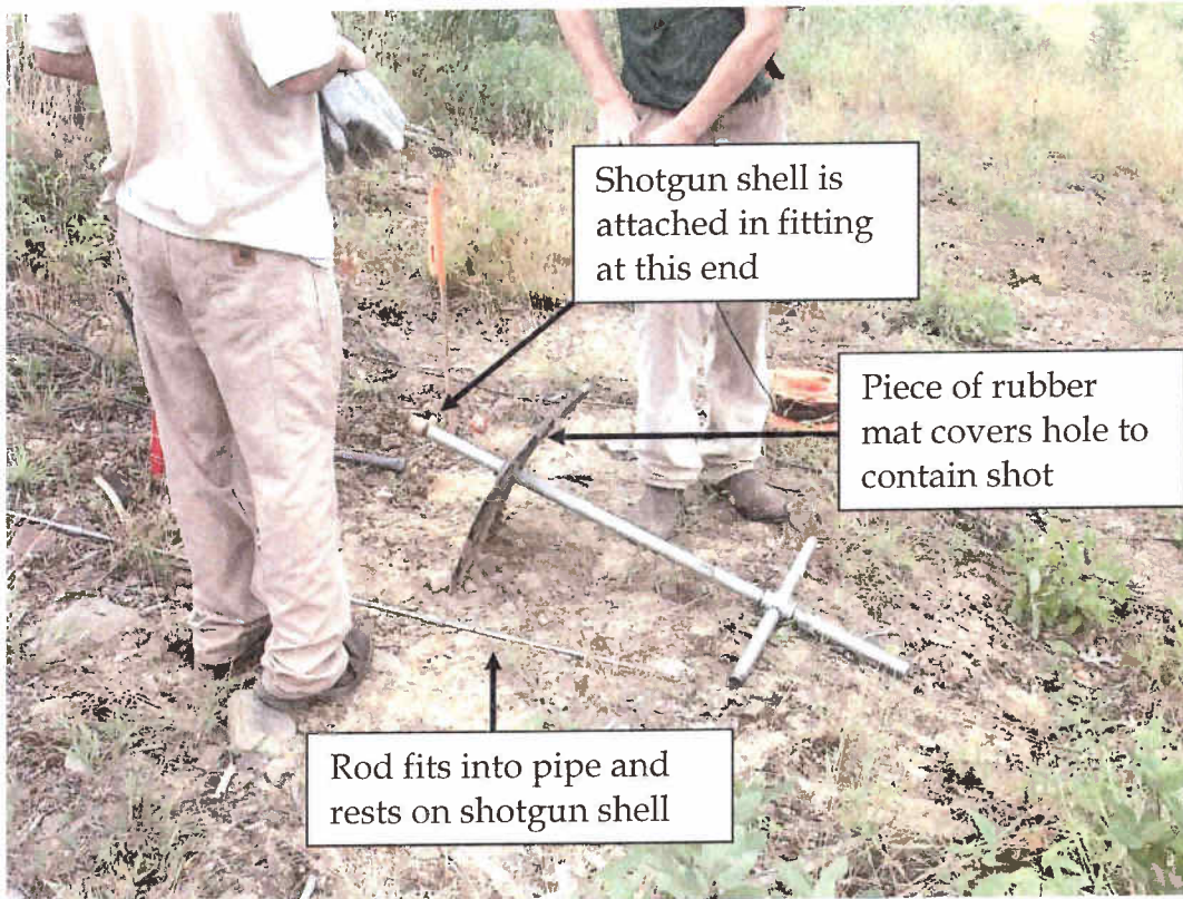
Figure 1: Overview of "seisgun" seismic source.
